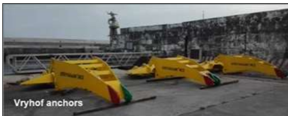
Figure 10. Drag Embedment Vryhof anchors utilized (Source: Tecnalia).
